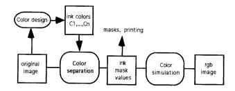
*Figure 1. The diagram of designing and simulation process of textile materials printing.*
